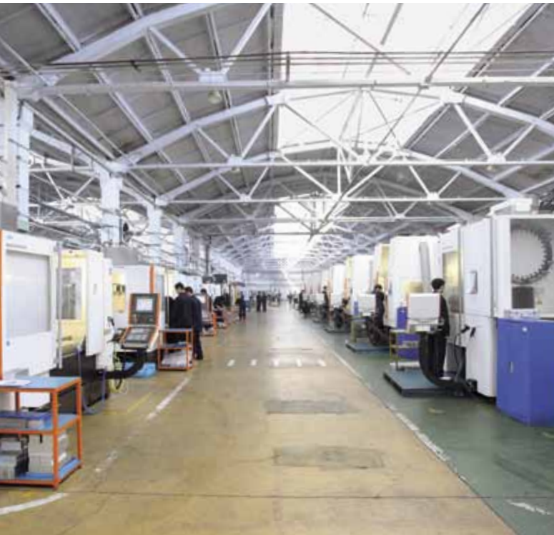
Successful partnership: HFIC works with 16 high-precision machine tools from GF AgieCharmilles to produce demanding aluminum helicopter components.
